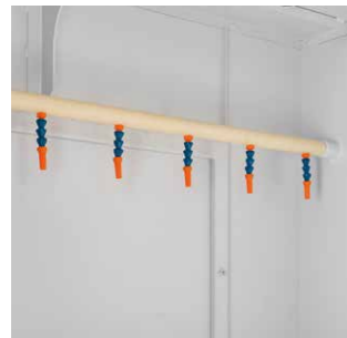
Chip shower Chip shower pipes are located at the upper section inside the machine for more efficient flow, and flexible shower nozzles can be directed to the side of the machine cover or sections where chips tend to accumulate.
