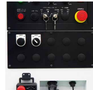
Switch panel (8 holes or 10 holes) Various switches, such as automatic door open/close switches, are set in specific locations. The switch panel (8 holes) is also available so that the position of the manual pulse connector can be changed.
