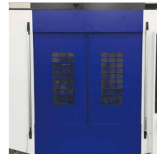
Area sensor Optical area sensors are used. Use area sensors to prevent operators being caught in the automatic door.
