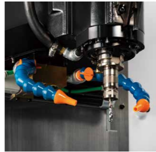
Head coolant nozzle Coolant can reliably be applied to the machining section as the tool and nozzles are set in place.
