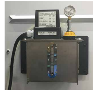
Automatic oil lubricator Regularly applies oil to all lubricating points on the three axes. * Manual greasing is required for the standard specification model.
