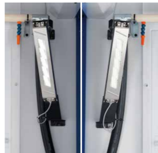
Work light (right side, left side) LED lamps are used to extend lamp life and save energy.
